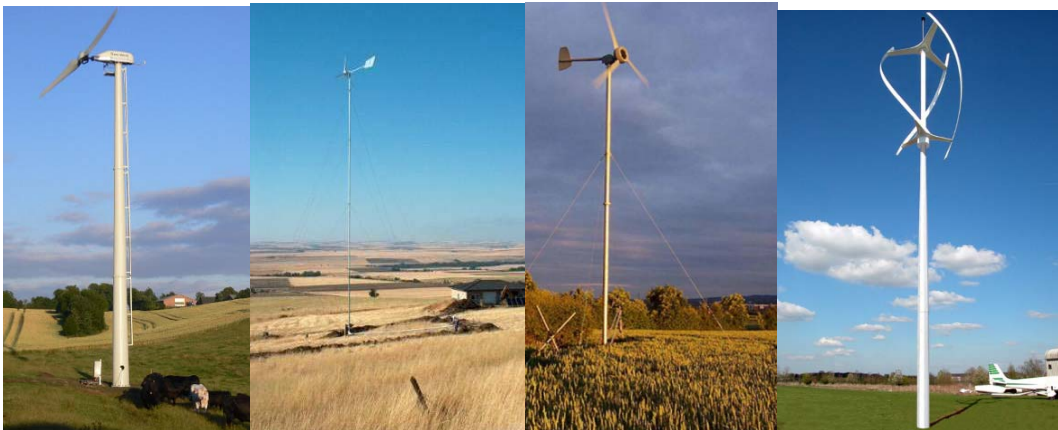
Figure 24, Examples of 5kW to 11 kW systems
